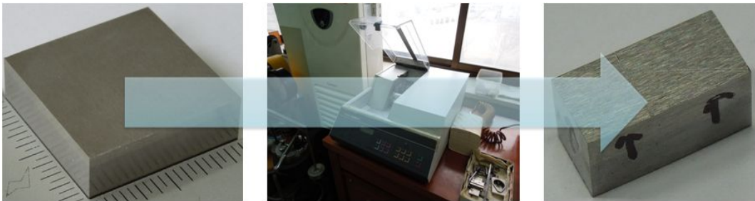
Fig. 24 Procedure of specimen fabrication for hardness experiments in the elevated temperature
