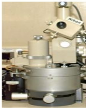
Fig. 25 High temperature vickers hardness tester (NIKON QM-2)
