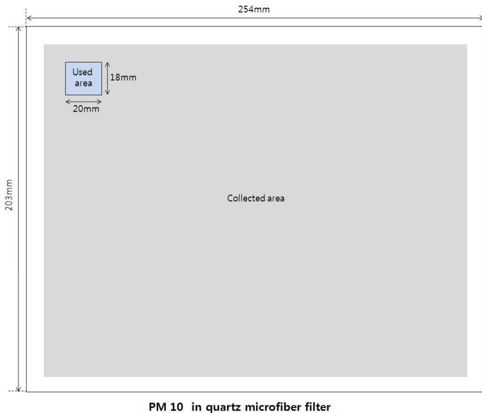
Figure 6. PM 10 sample amounts applied to internal TD-GC-MS system
