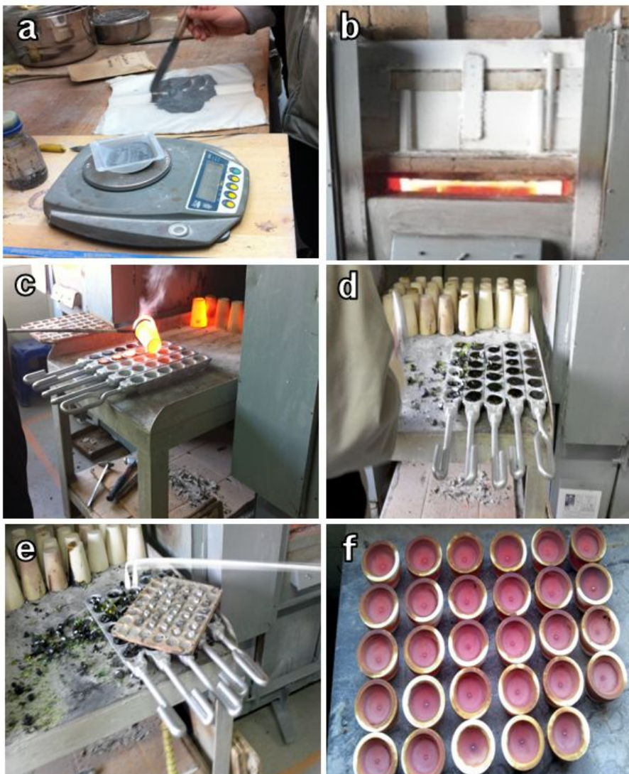
Figure 7. The method of lead-fire assay analysis in this study (a; weighting of fusion flux, b; fusion, c; molding, d; separation of glassy slag, e; cupellation, f; silver beads in the bone ash crucible).
