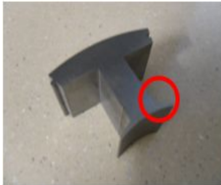
Photo 5.3 HV hardness test zone of core part
