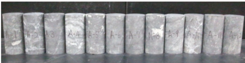
Figure 4-2. Core specimens for physical tests in laboratory, (a) pyrrhotite, (b) ilmenite and (c) magnetite.
