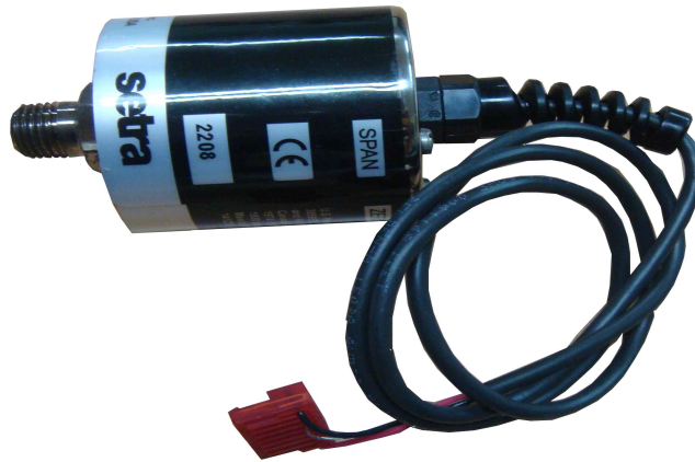
Fig. 2.6 Photograph of pressure gauge.
