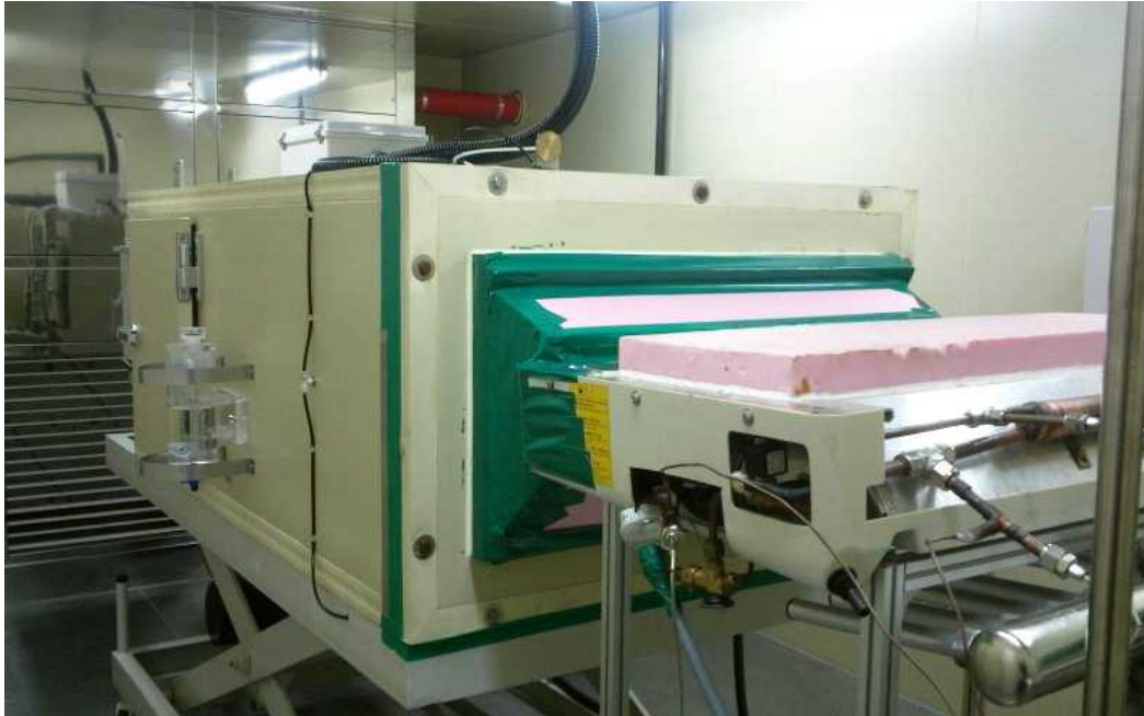
Fig. 2.13 Calorimeter with an evaporator.
