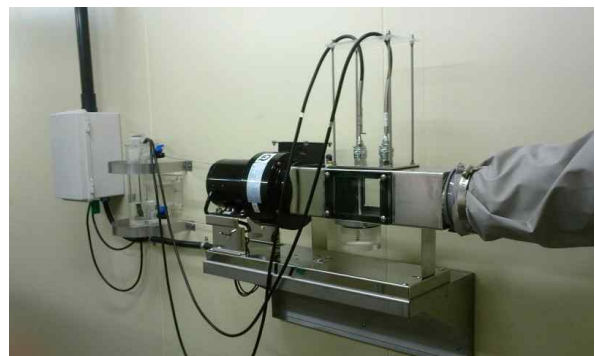
Fig. 2.11 Air sampler and blower.
