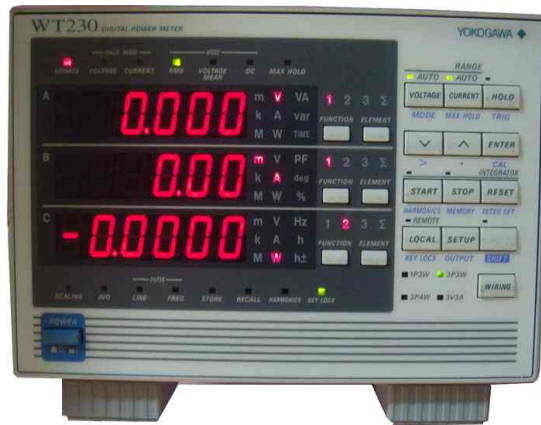
Fig. 2.8 Photograph of power meter.
