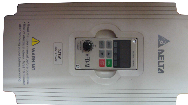
Fig. 2.7 Photograph of inverter.
