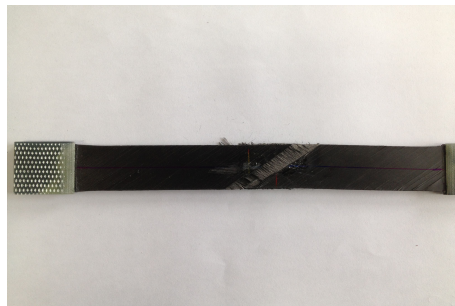
Fig. 3.2.2.8 Failure of specimen [\pm 45^\circ]_{10}
