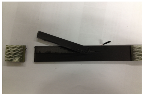
Fig. 3.2.2.12 Failure of specimen [0^\circ / 90^\circ]_{10}
