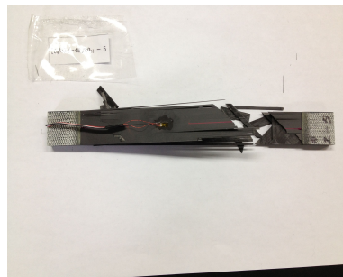
Fig.3.2.2.6 Failure of [0_4/+45_6/-45_6/90_4]_s
