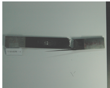
Fig.3.2.2.9 Failure of [0_5/+45_5/-45_5/90_5]_s
