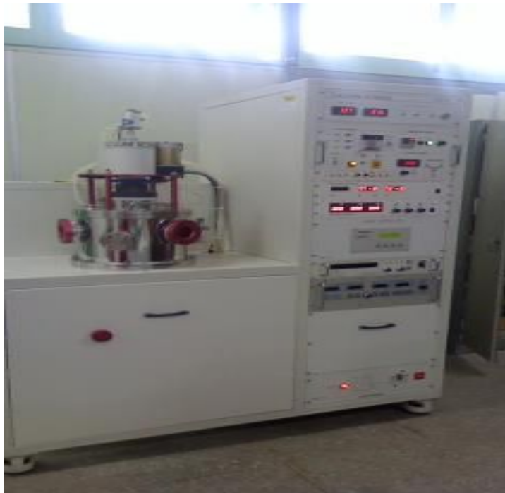
Fig.9 Sputter equipment (Vacuum Science Co.)
