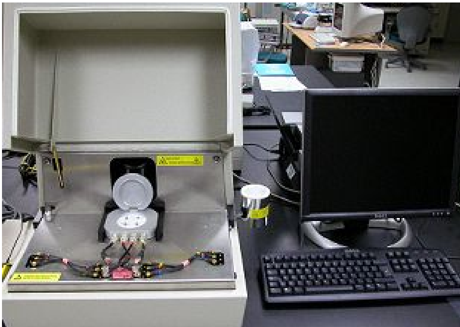
Fig. 14 Hall Effect measurement system equipment (Accent Optical Technologies. HL5500PC)
