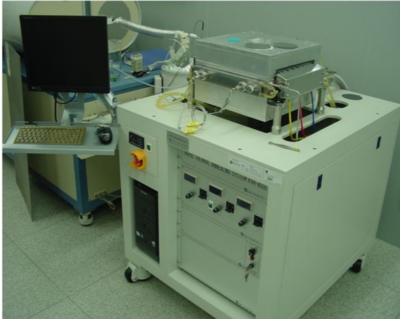
Fig.10 Rapid thermal annealing equipment (Modular Process Technology Co., RTP-600S)
