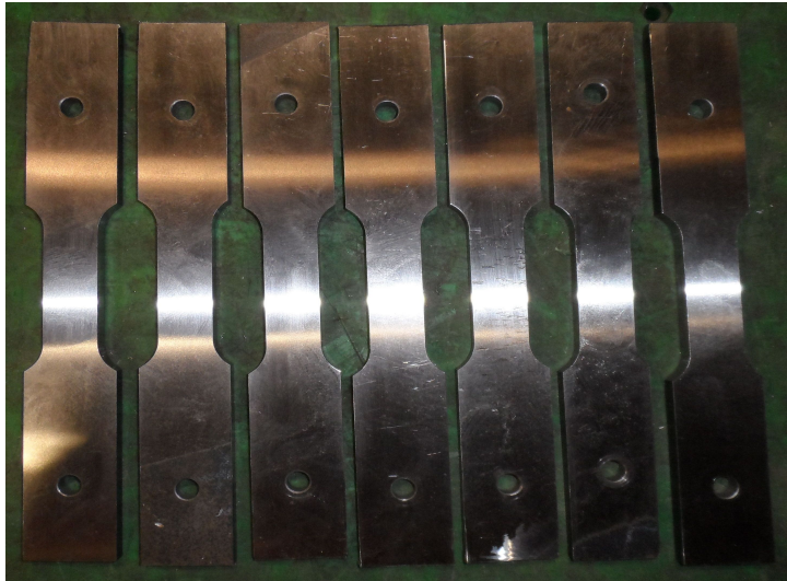
Fig. 3-10. After fine grinding of tensile test specimens
