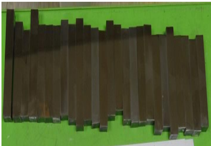
Fig. 3-12. After fine grinding of hardness test specimens
