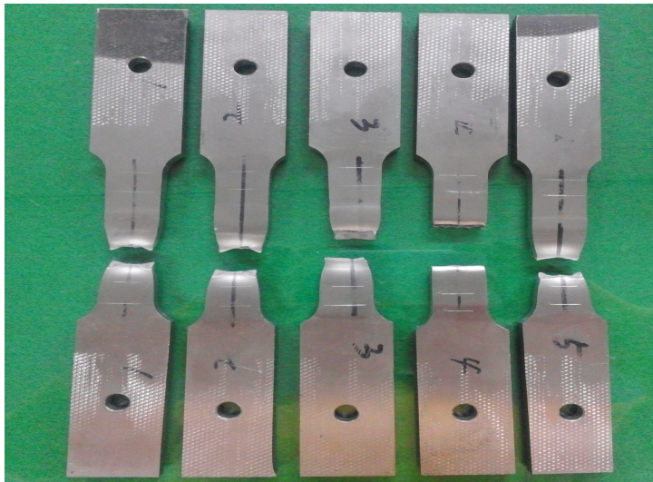
Fig. 3-11. After tensile test of specimens
