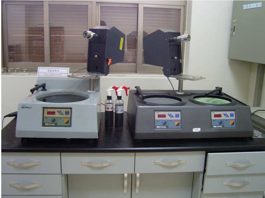
Fig. 3.5 Automatic Grinder / Polisher
