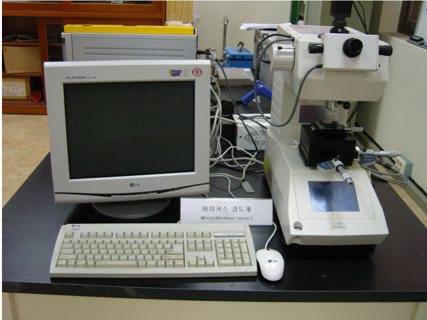
Fig. 3.7 Micro Vickers Hardness Tester
