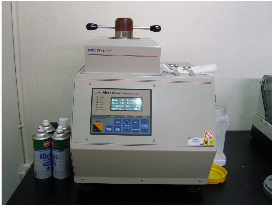
Fig. 3.4 Hot mounting press
