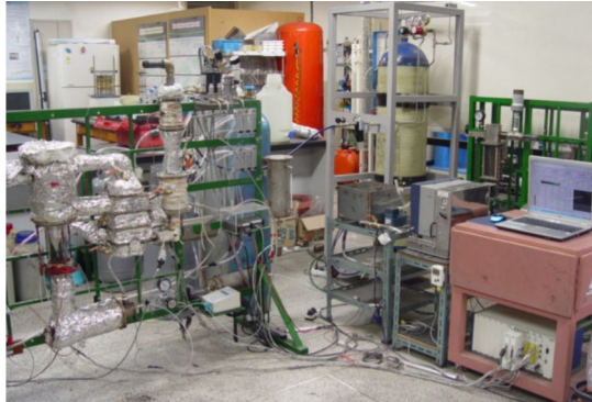
Fig. 5-2. Photo of a hydrogen-rich gas production system.
